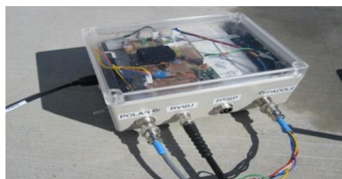
Figure 3.3-3: Analogue to digital converter collecting data from strain gauged paddle.
