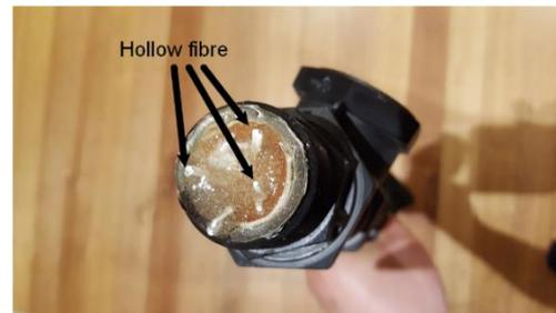
d) hollow fibre packing density (top view)
