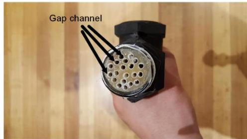
b) gap channel density (top view)
