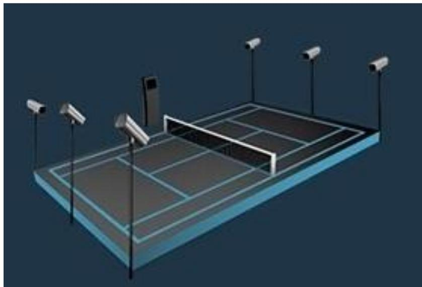
Figure 5.1: Tennis court equipped with Playsight system with 2 HD cameras and 4 analytical cameras
