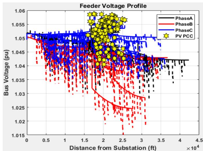
Fig. 3.6. Voltage profile with PV system at CKT24.
