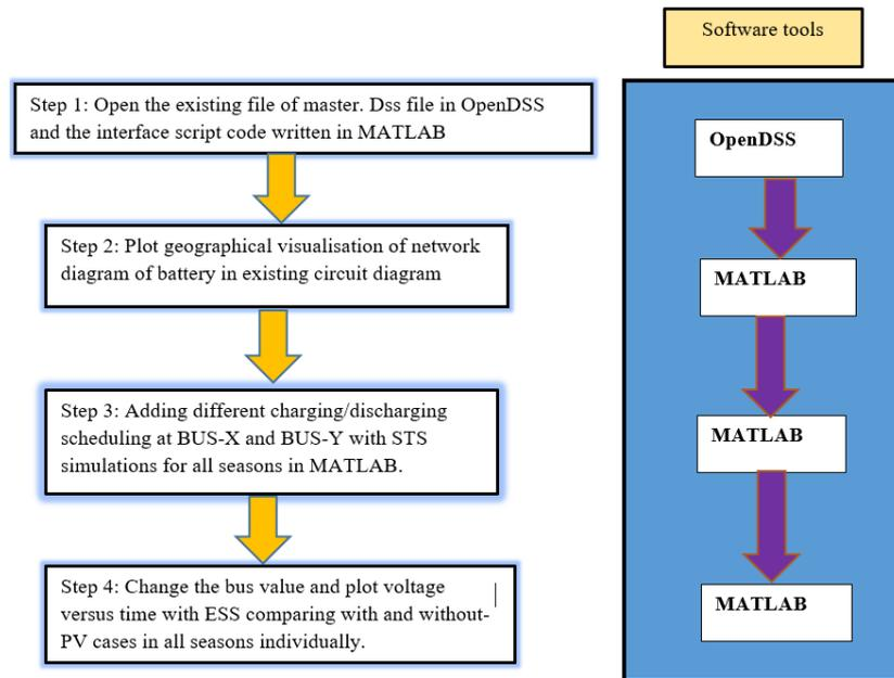
Fig. 4. 2. Detailed toolchain level of seasonal ESS.
