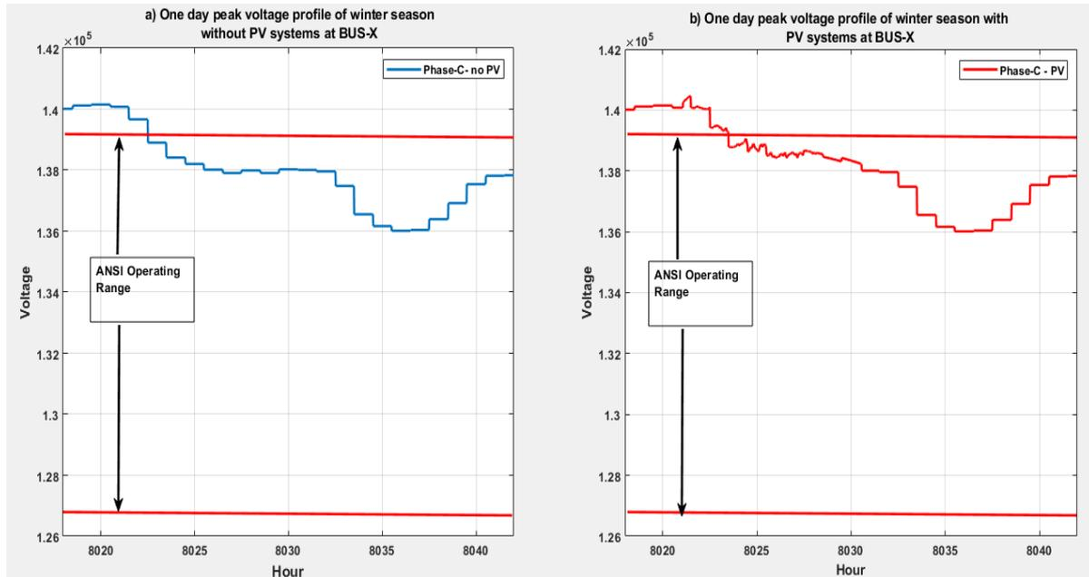
Fig. 3.11. Daily voltage profile in winter season with and without PV systems at BUS-X.
