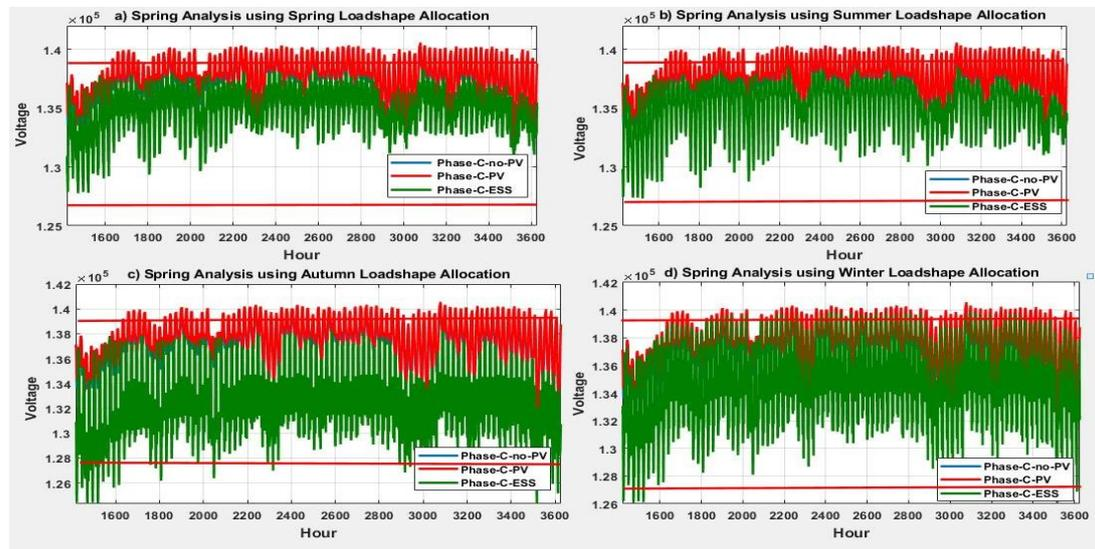
Fig. 4. 15. Spring season analysis using different seasonal LoadShape allocations at BUS-X.
