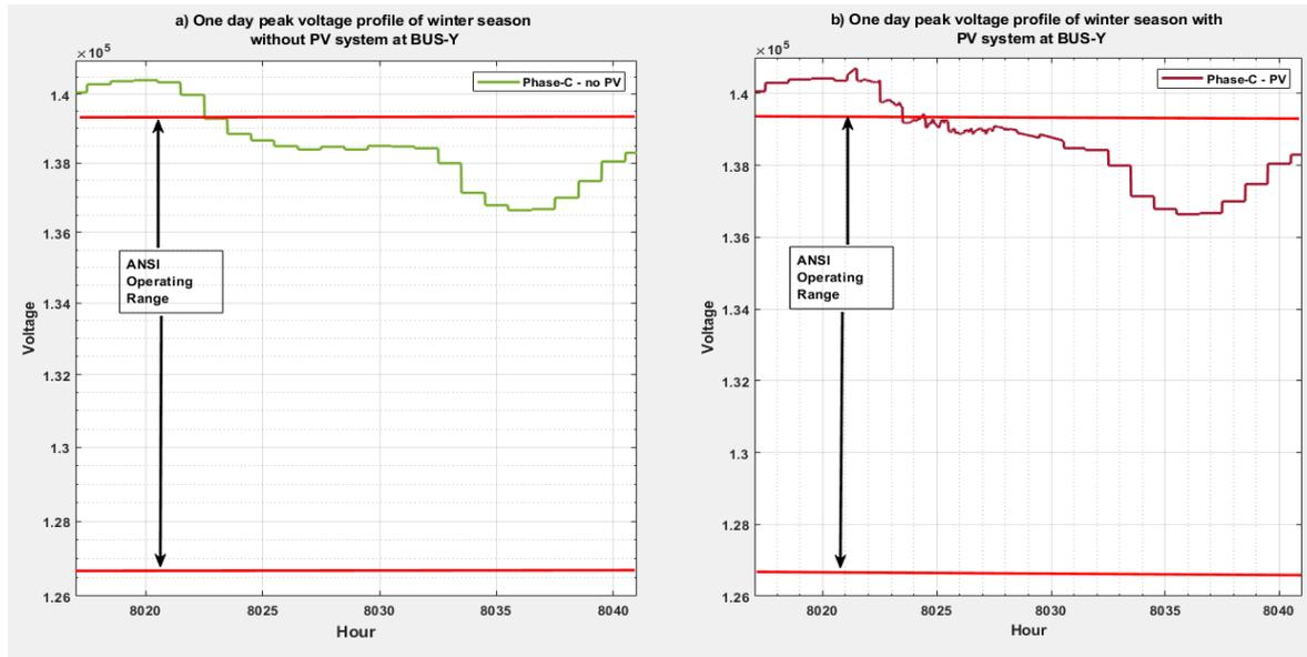
Fig. 3.16. Daily voltage profile in winter season with and without PV system at BUS-Y.
