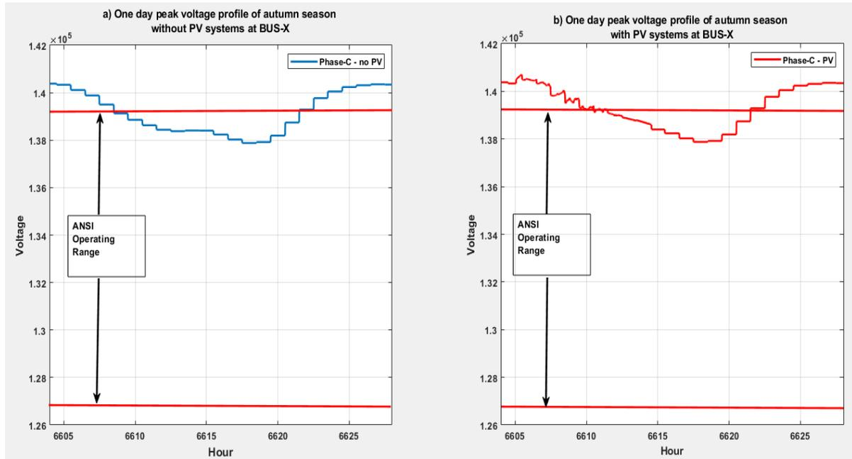
Fig. 3.10. Daily voltage profile in autumn season with and without PV systems at BUS-X.
