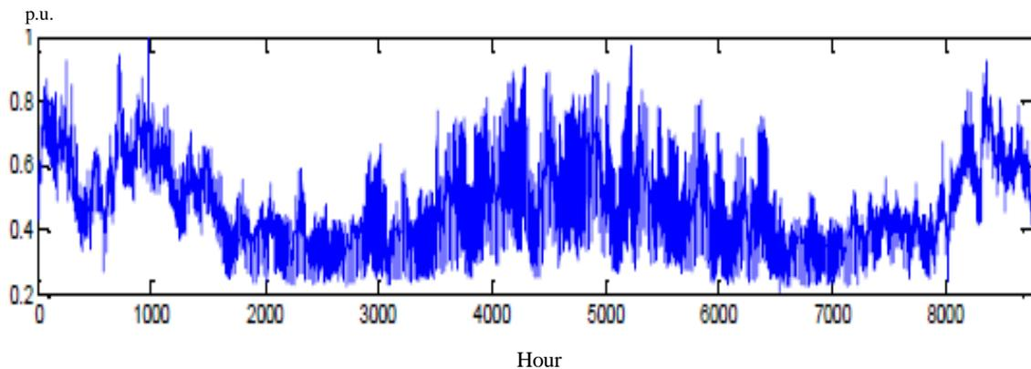
Fig. 3.3. Average Three Phase EPRI CKT24 load shape for one year [81].
