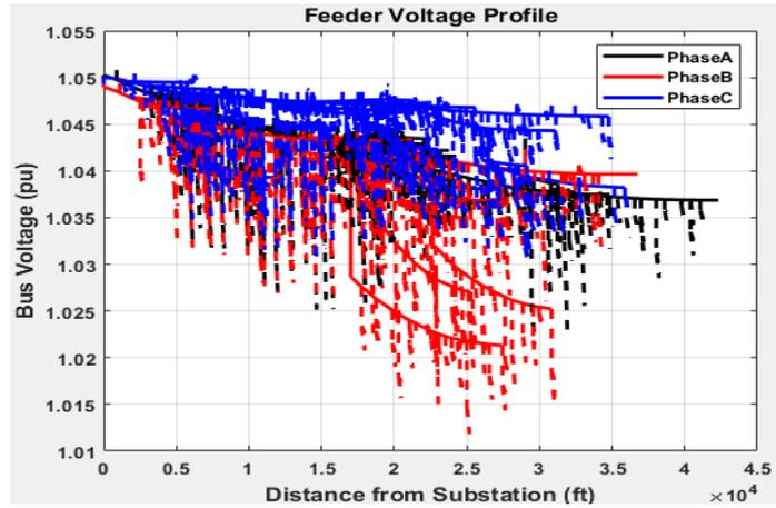
Fig. 3.5. Voltage profile with No PV system at CKT24.
