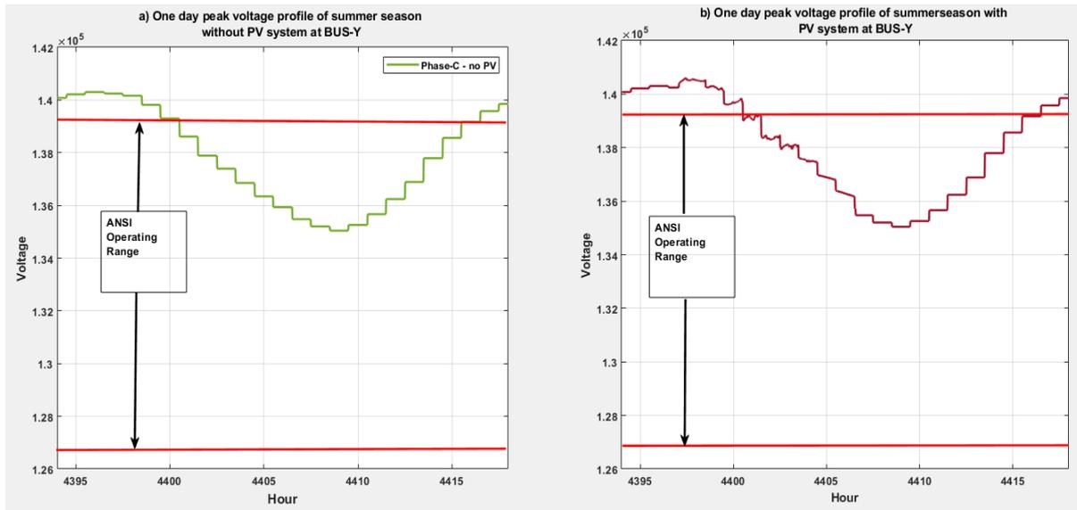
Fig. 3.14. Daily voltage profile in summer season with and without PV system at BUS-Y.
