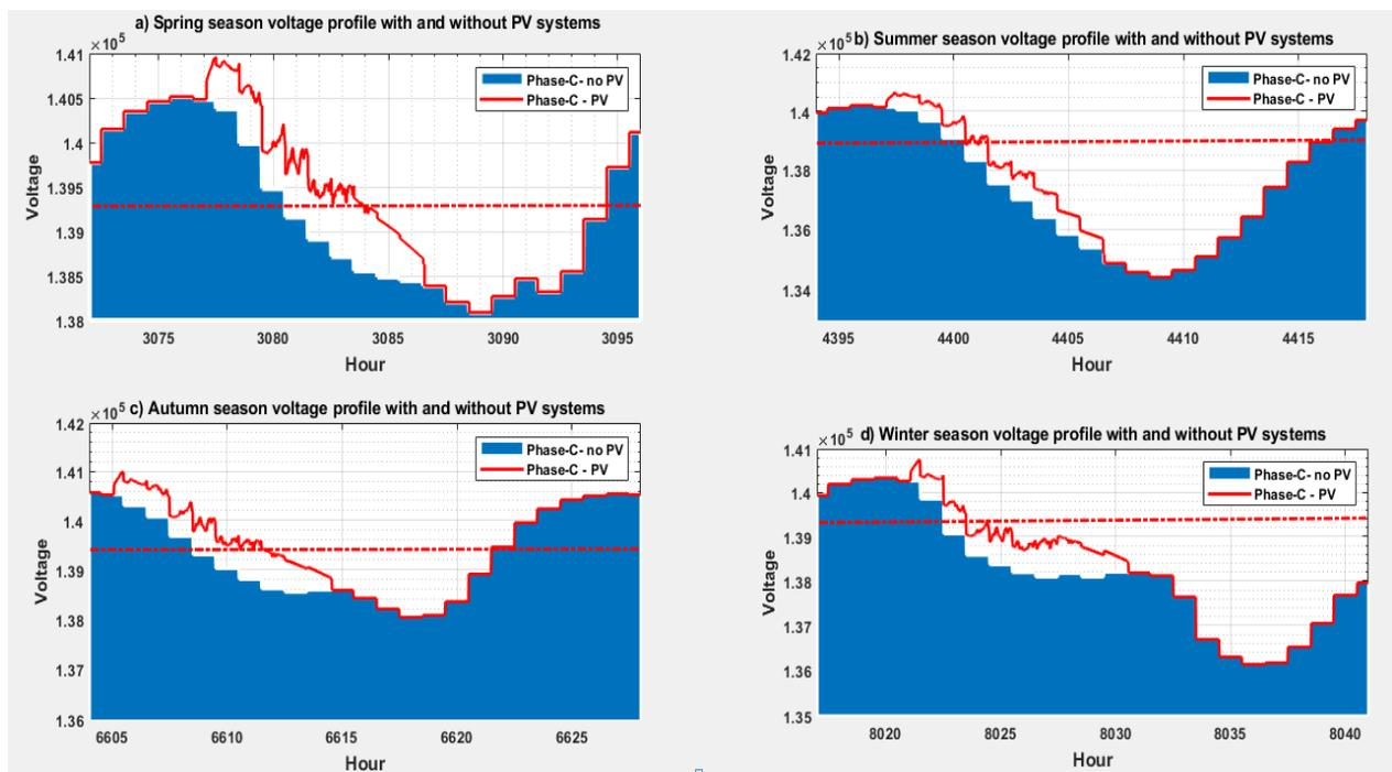
Fig. 3.12. All seasons one-day peak voltage profile with and without PV systems at BUS-X.
