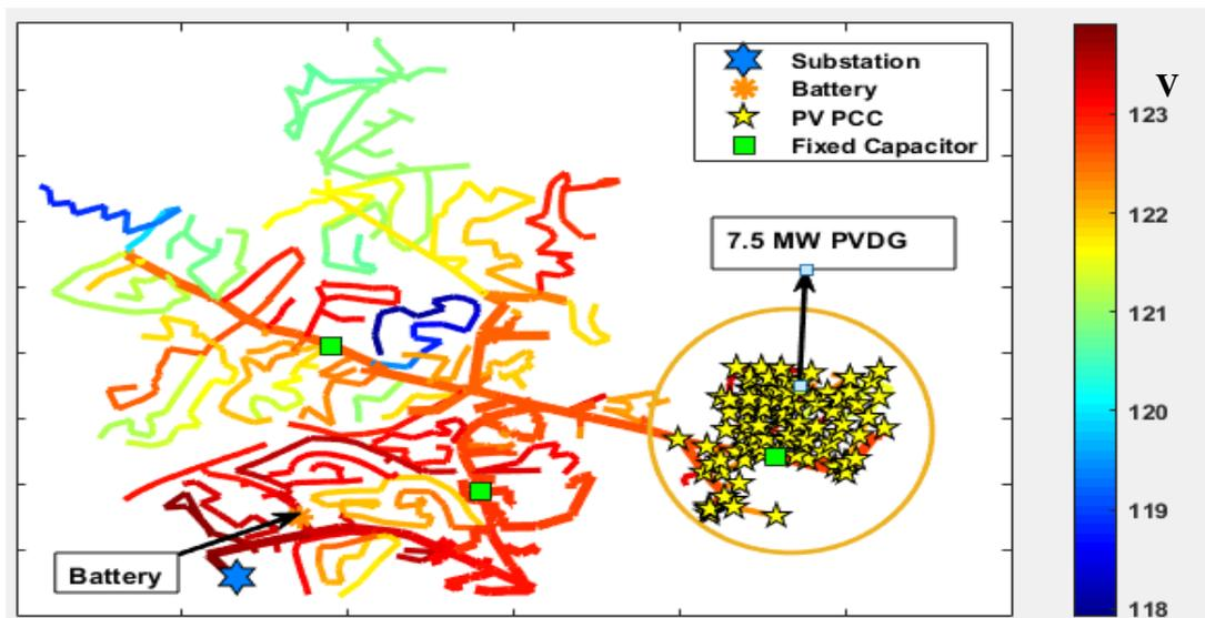
Fig. 4. 9. Simulation results of grid integrated PV/Battery network diagram of CKT24 at BUS-X.
