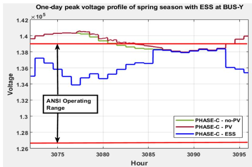
Fig. 4. 18. Seasonal scheduling of charge/discharge dispatch in the spring season at BUS-Y.
