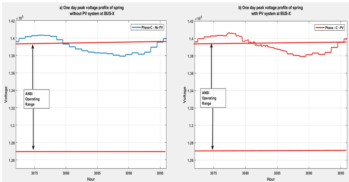
Fig. 3.8. Daily voltage profile in spring season with and without PV system at BUS-X.
