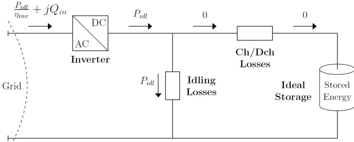
Fig. 4. 6. The Operation of a storage element in a discharge state [101].
