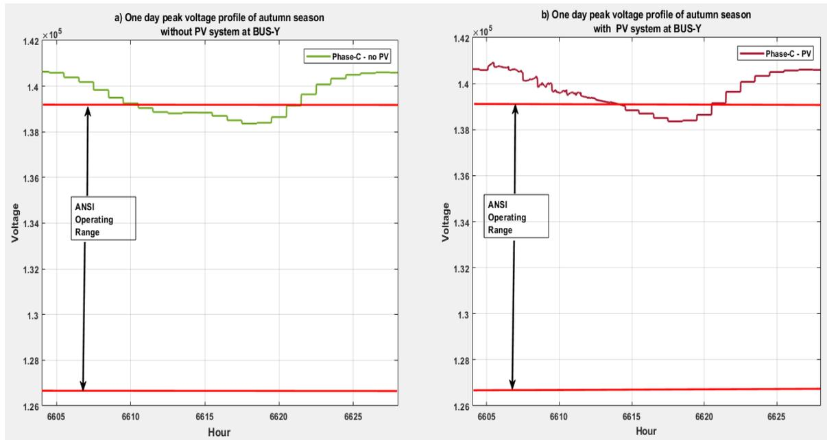
Fig. 3.15. Daily voltage profile in autumn season with and without PV system at BUS-Y.
