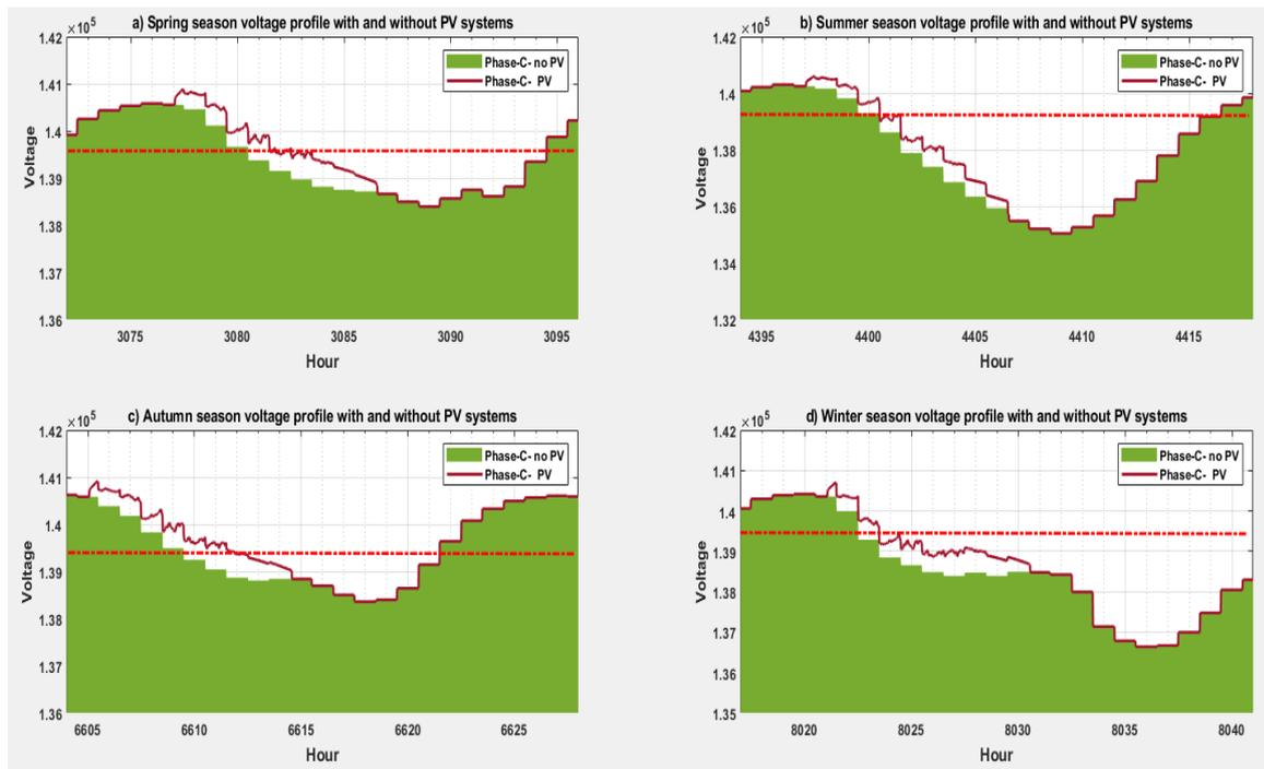
Fig. 3.17. All seasons one-day peak voltage profile with and without PV systems at BUS-X.
