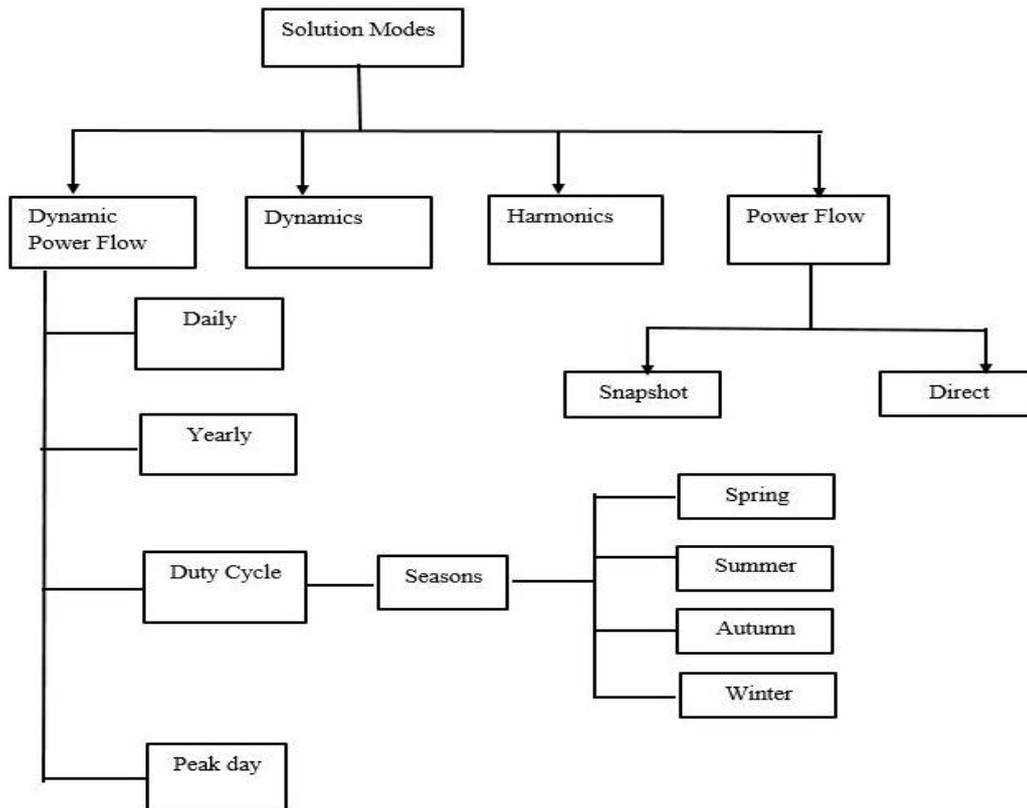
Fig. 1.4. Different solution modes accessible in OpenDSS.
