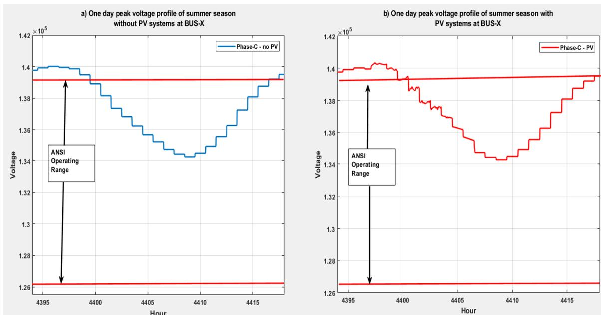
Fig. 3.9. Daily voltage profile in summer season with and without PV systems at BUS-X.
