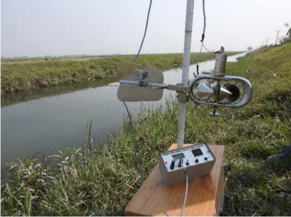
Figure 8.1: Current meter used for discharge measurement in the main irrigation canal.
