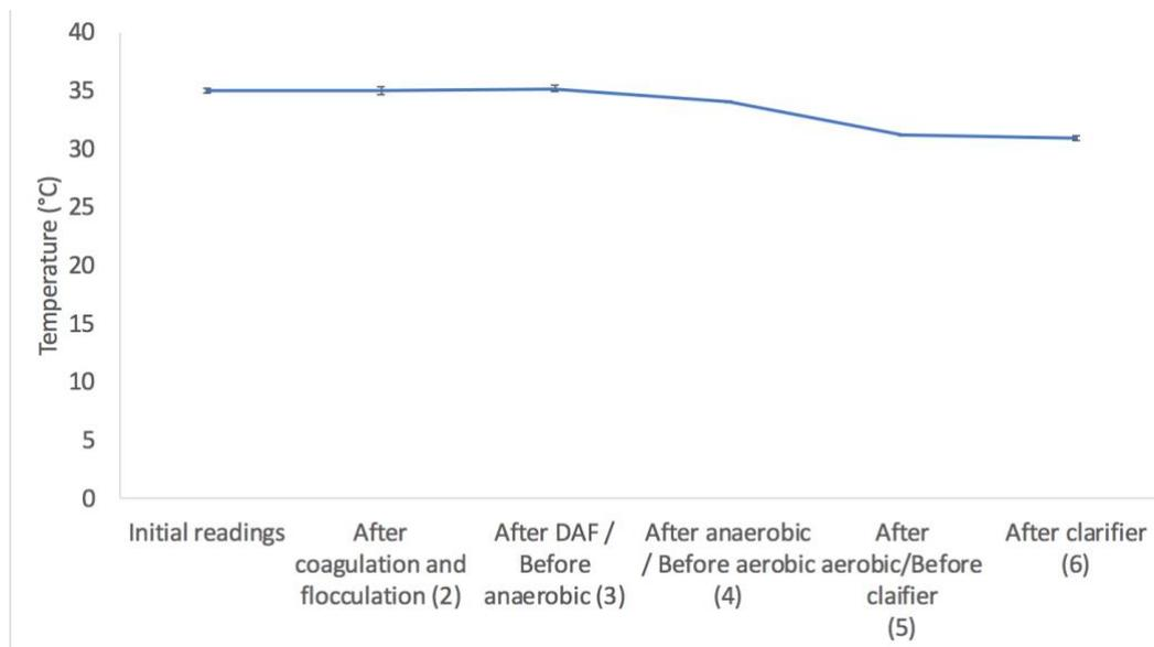
**Figure 4.9.** Temperature values at each point of the wastewater treatment process.
