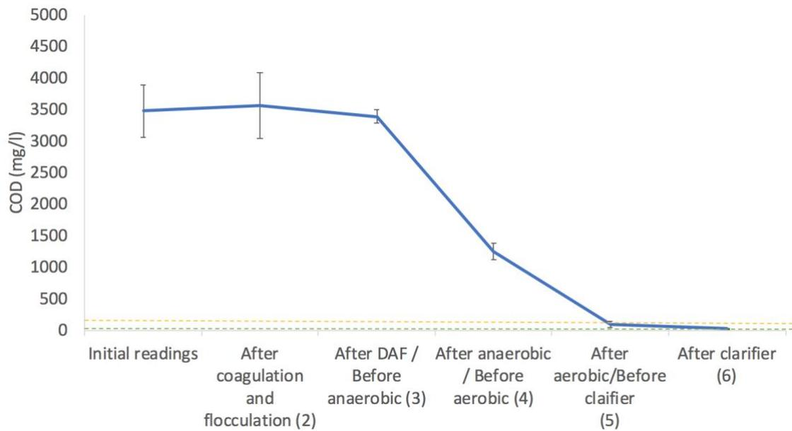
**Figure 4.4.** COD values at each point of the wastewater treatment process.
