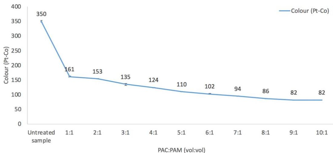
**Figure 5.2.** Colour removal efficiency of different PAC:PAM (vol:vol) ratios given a fixed amount of PAM and an increasing amount of PAC.
