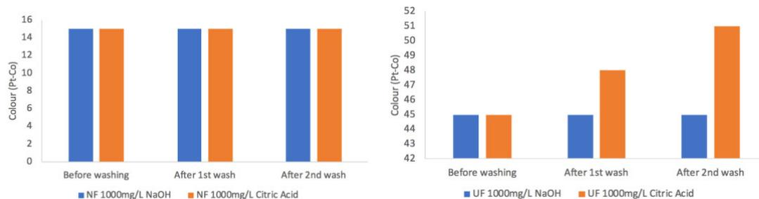
**Figure 6.6.** Colour removal of NF (left) and UF (right) being cleaned with 1000 mg/L NaOH and citric acid (Feed colour = 1343 Pt-Co)
