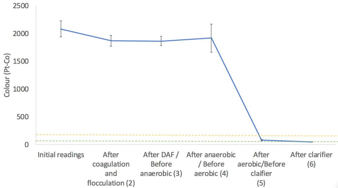
**Figure 4.5.** Colour values at each point of the wastewater treatment process
