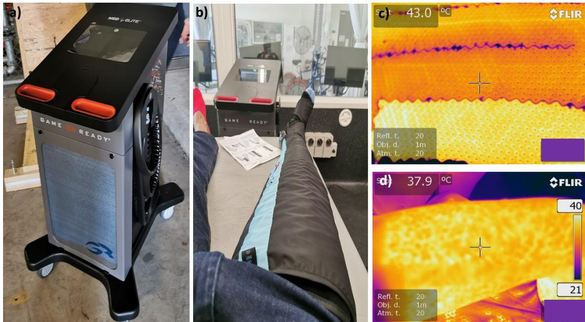
**Figure 2.5.** a) The Med4elite™ heat, cold, contrast and compression therapy platform by Game Ready®. b) The full leg boot applied in a testing session, c) the infrared profile of the wrap closer to maximum temperature. The water is guided through by sewn in seals which are visibly much colder, d) the thermal profile of the quadriceps 60 seconds after the removal of the wrap. The homogenous heating is evident.
