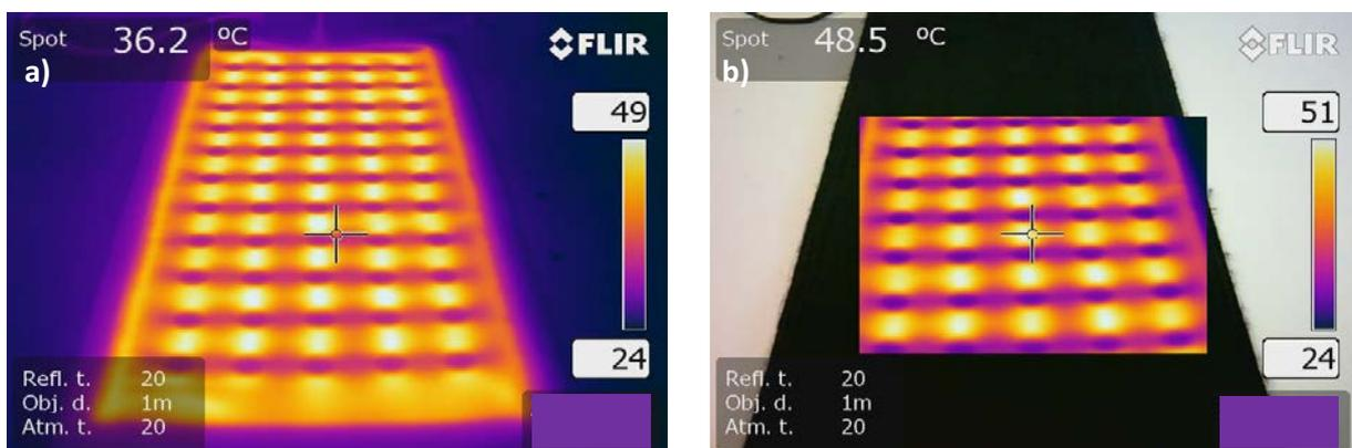
Figure 2.3. FLIR® infrared images of the Exo2® heat wrap; a) full scale infrared image b) sectional image. Cross hairs aimed at heating element (or chain) in image (b).
