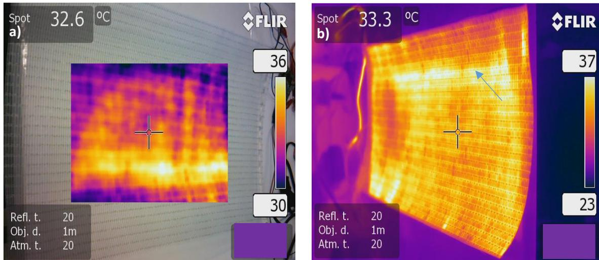
**Figure 2.4.** a) The FLIR® infrared images of SEFAR® PowerNT™ heat mesh. The hotter area depicted in b) was caused by the mesh being less in contact with its resting platform.
