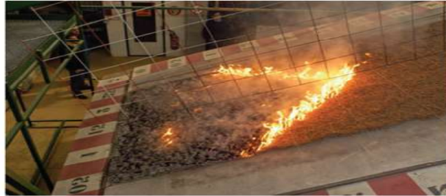
(a) Fire-front view from the experimental study of Dupuy et al. (2011): +20°, 2 m wide fuel bed
