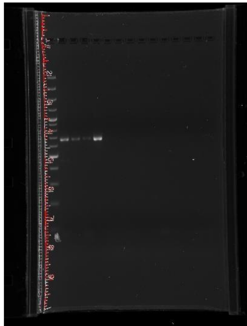
Figure 10.6b. Bioanalyser results on the gel (the first lane from left shows the DNA ladder bands, the next 4 lanes are samples)
