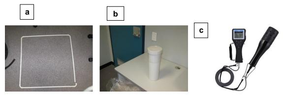
**Figure 2.6: (a)** 50 cm X 50 cm Quadrat used to randomly find sample – Source: own image; **(b)** 10 cm internal diameter by 26 cm length of PVC pipe used to collect seagrass and sediment sample – Source: own image; **(c)** Horiba U-50 – Source: <u>https://www.horiba.com/en\_en/products/detail/action/show/Product/u-50-434/</u>
