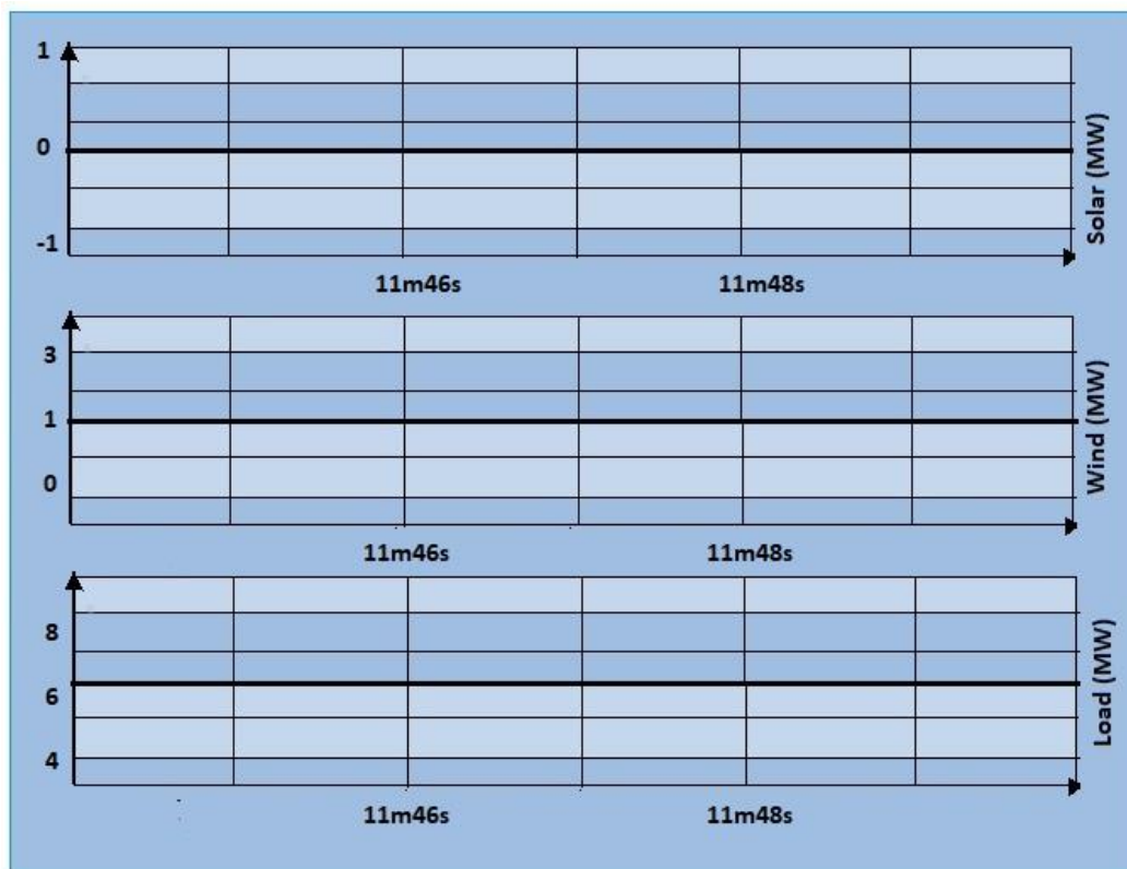
Fig 6.14 System performance when load demand is more than generation and battery reaches minimum state of charge
