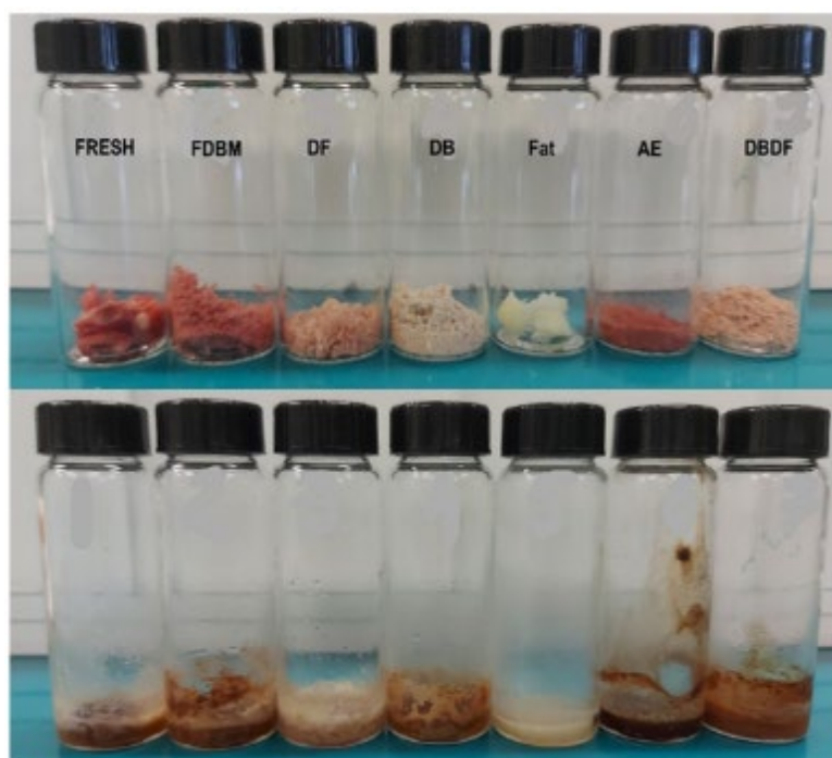
Figure 4.2 Before and after heat treatment (in vial 160°C- 30 min) of rehydrated FDBM fractions prior to HS SPME-GCMS analysis.
