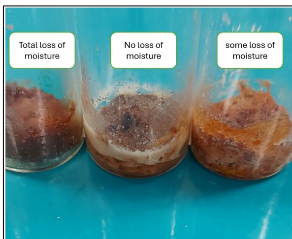
Figure 3.4 Varying degrees of moisture loss from the vial due to pressure build-up during heat treatment in an oil bath.
