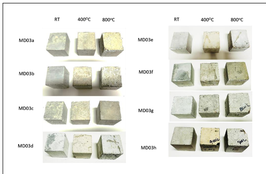
Figure 4.48: Physical appearances of MD03 a-h specimens at room temperature, and after exposure to 400°C and 800°C
