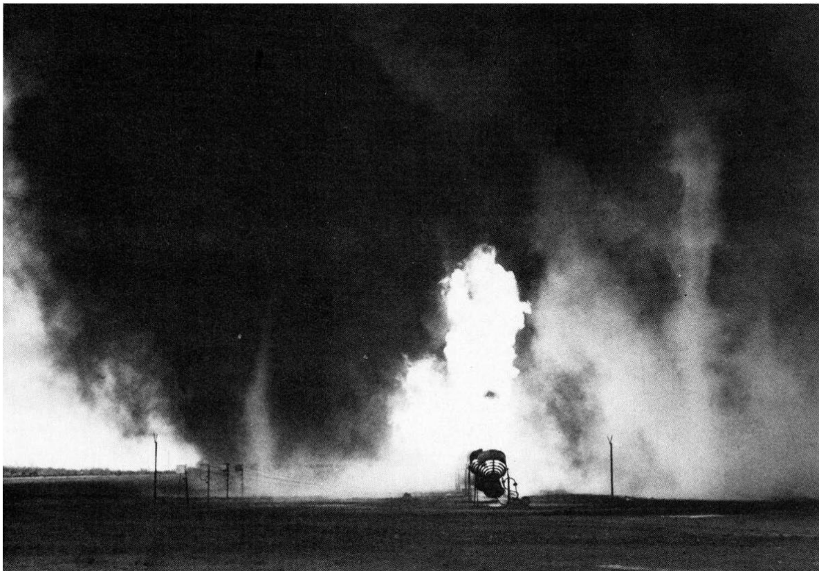
Figure 5-5: Paired wake vortices on either side of a fuel burner heat source. The vortices are rotating in opposite directions – the vortex on the left showing cyclonic rotation and the vortex on the right showing anticyclonic rotation. Source: Church, Snow and Dessens [82]
