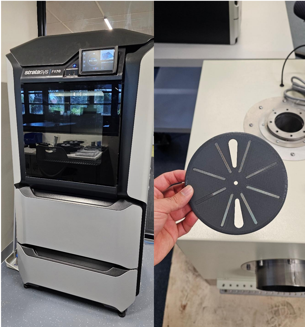
Figure 4.8. The picture on the left shows F170 printing the disks. The printed bottom part of the disk is shown in the picture on the right.
