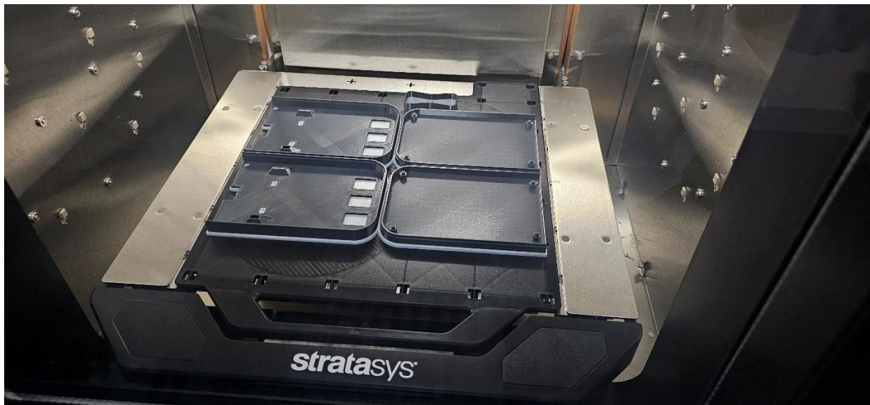
Figure 3.49. Printed cases on Stratasys F170 plate. The case (grey) can be seen made of ABS (Acrylonitrile Butadiene Styrene) plastic, on a white layer of QSR (Quick Support Removal)
