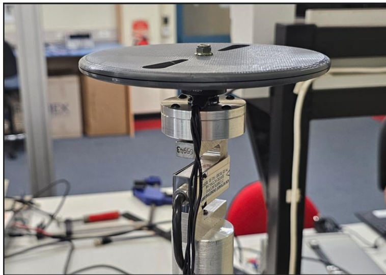
Figure 6.6. The S-Type Load Cell Scale Sensor installed in line with the hybrid Validist Encoder disk.
