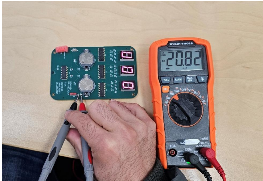
Figure 5.13. The circuit's current measurement for power consumption assessment.
