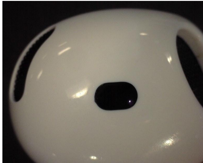
Figure 6.3. The proximity sensing system based on reflecting a modulated IR signal to detect if the AirPods 4 is worn by the user. The Activated IR beam is visible on the bottom right-hand corner of the black oval shape.
