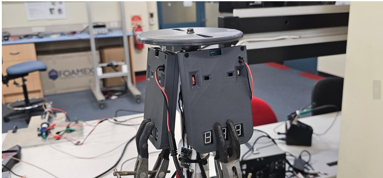
Figure 6.1. The hybrid encoder system (Validist Encoder) with the optical sensing on the left and the magnetic sensing on the left.
