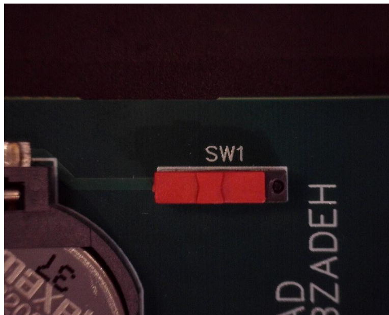
Figure 3.21. The slide switch on the board.
