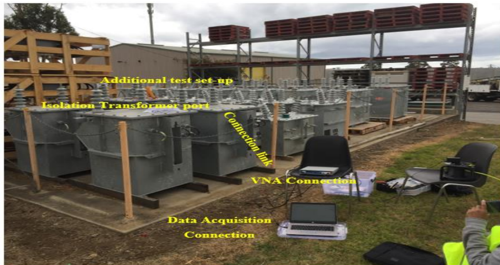
Fig 5.31: SWER isolation transformer data acquisition set-up
