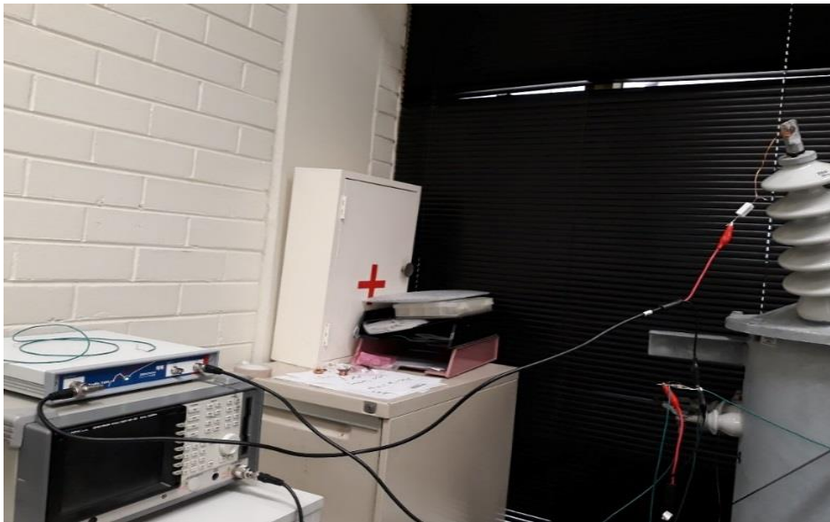
Fig 5.13: Experimental arrangement for the Touchstone file acquisition
