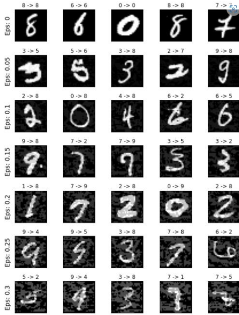
Figure 5. 2 FGSM attack on MNIST showing the intensity (less aggressive) on varying epsilon
