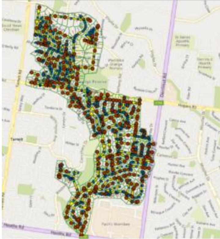
Figure 4.7. 2022 Overflowing Manholes Identified Based on Flood Volume and Flow Rate
