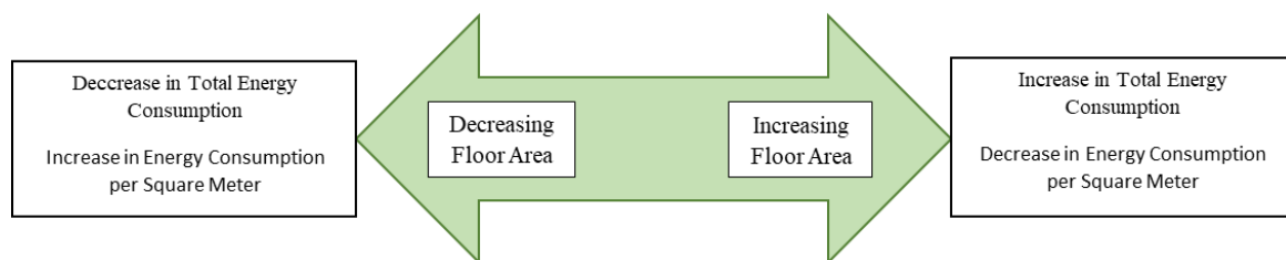
Figure 5-1. Analysis of the Impact of Floor Area on Energy Performance Based on Results
