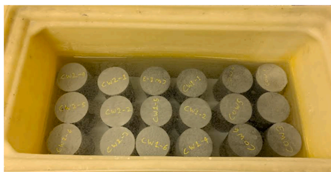
Fig. 2. Setup and curing of concrete samples.
