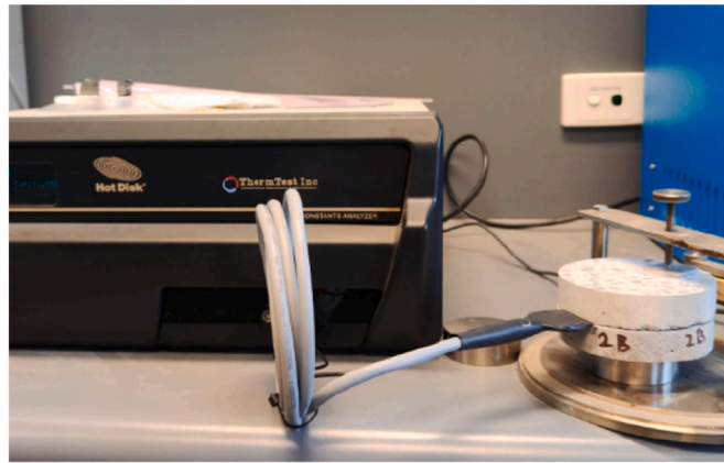
Fig. 3. Thermal conductivity tests on the samples.
