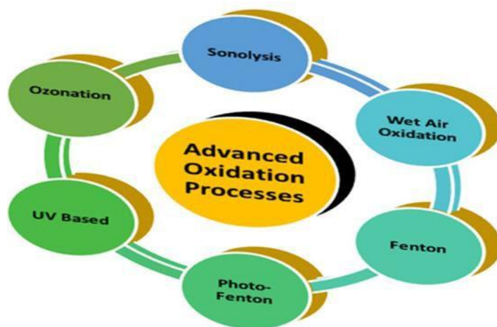
Figure 1. Classifications of advanced oxidation process (Adapted from Mishra N. S, 2017).
