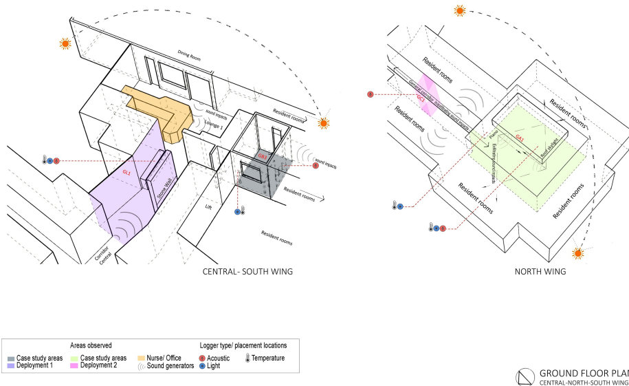
Figure 3. Potential for solar gains near skylight area GA1 (near piano) in the Phase 1 facility (now demolished). The diagram and legend show Phase 1 logger locations and types (acoustic, light and temperature) in bedroom (GB3), communal spaces (GA1 and GL1) and transition space (GC1)
