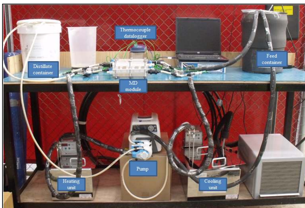
Figure 3.2 Bench-scale DCMD apparatus.
