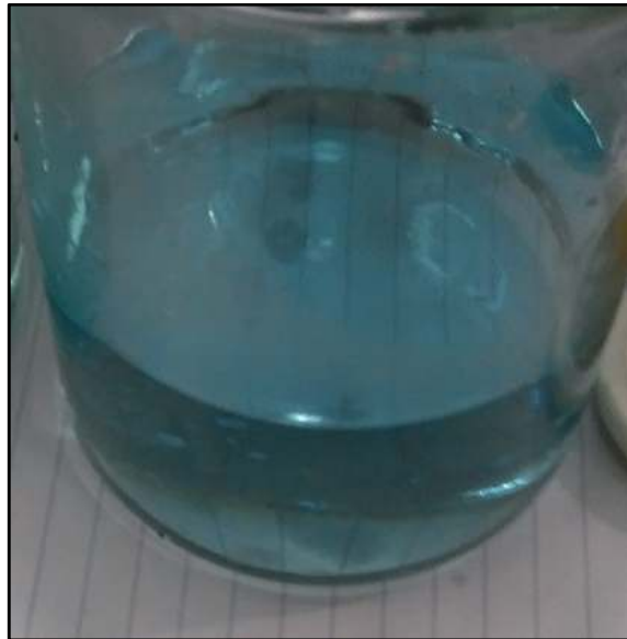
Figure 3.7 Copper barren RO brine.
