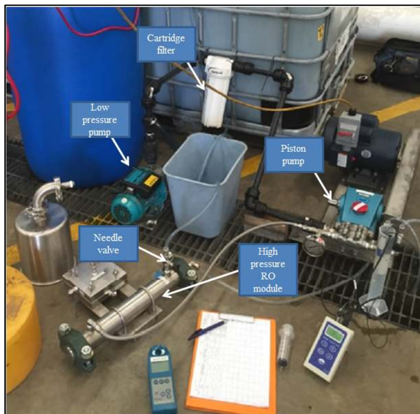
Figure 3.6 Bench-scale UHP RO apparatus.
