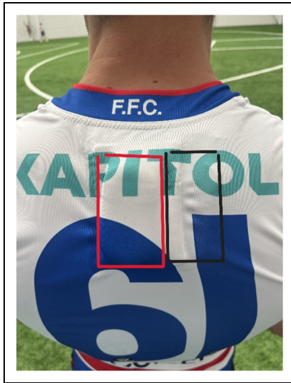
Figure 1. Placement of GNSS units in the football training jumper and custom sports vest. The Vector S7 unit is marked in red and the K-AI unit in black.
